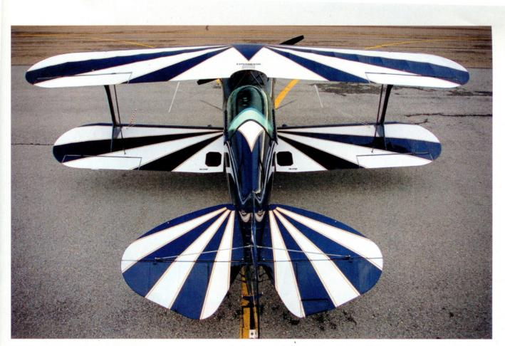
A hand-painted emblem on the vertical stabilizer shows pride in the designer (lower left). The Pitts is an airplane the pilot "wears," and the cockpit (left) with a parachute and five-point harness is extremely confining. Four ailerons and a short wingspan give the Pitts a quick roll rate, and oversized control surfaces make it extremely maneuverable in every axis. The starburst paint scheme (above) matches the brash design.
